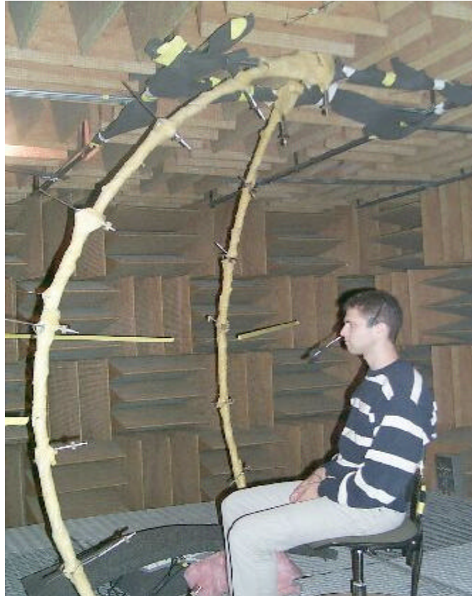
Figure 1: The array of microphones surrounding the subjects in the anechoic chamber.
